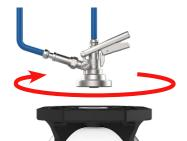
1. Insert the head turning it clockwise on the keg coupling.
