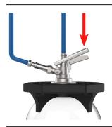
2. Couple the head by pushing down the lever.
